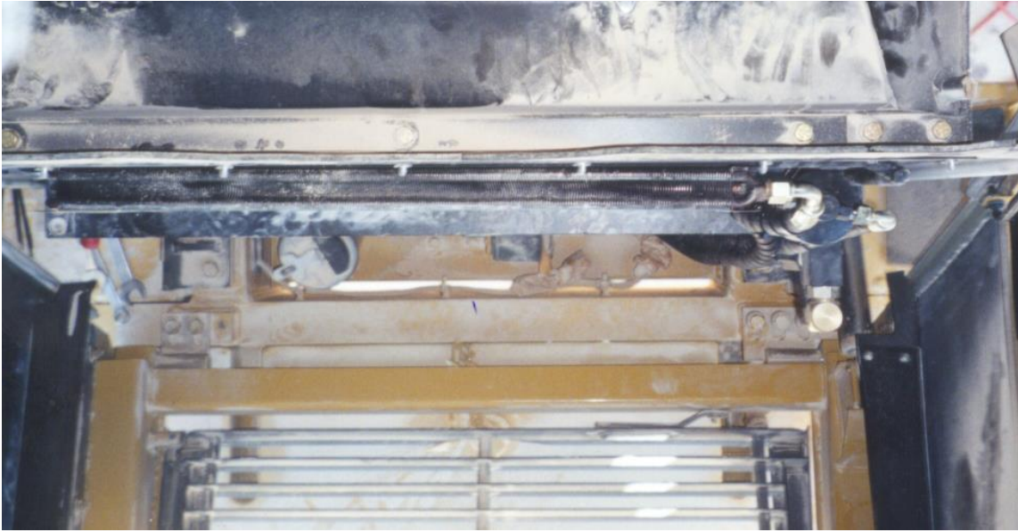
Top view of condenser mounted on outside (rear) of radiator assembly.
