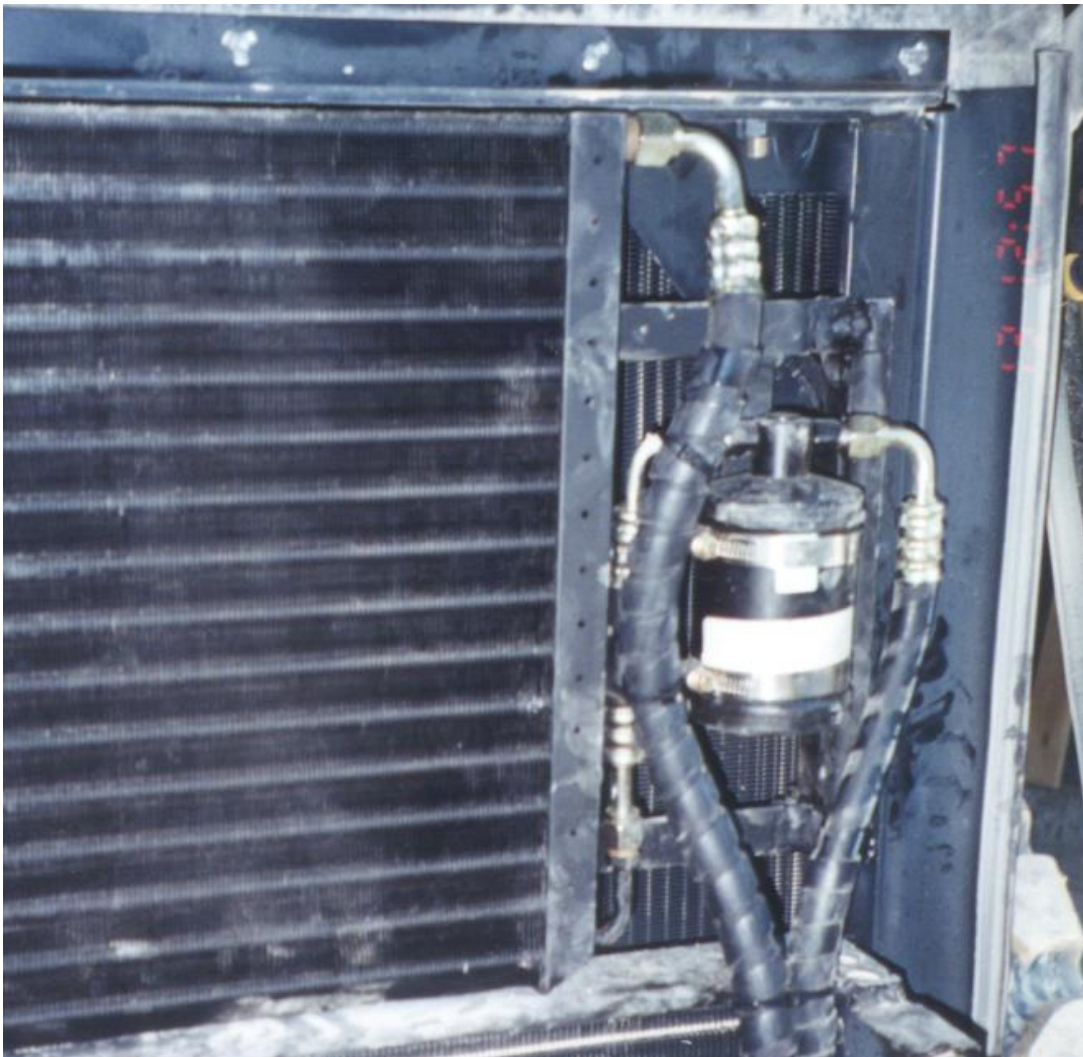
Right hand side of condenser assembly with drier and hoses.
